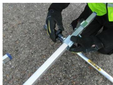
Screw the two Wheel screws into the sliding shoes.
