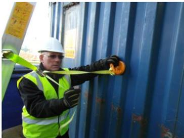
Keeping the strap horizontal attach the suction cup to a suitable glazed window. The above picture is for demonstration purposes only, usually the cup is positioned against the glass of a conservatory.
