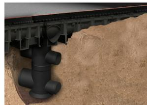
Lay channels starting from outlet/sump, ensuring joints connect by lowering units horizontally. Fit endcaps to end channels. For fully watertight joints, use a suitable sealant (contact ACO for further advice).
