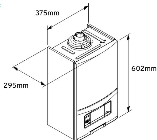
Note: A minimum of 600mm clearance in front of the boiler is required to enable easy access for servicing. This may be provided by an accessible door.
