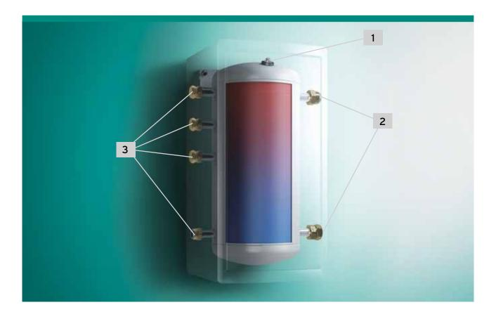
Should the system have multiple zones and/or require an additional pump to support the complete heating system, the decoupler module provides an excellent solution and is easy to site and install. The tank comes complete with an NTC sensor and pocket at the top of the tank as well as an air bleed valve/vent to help remove air from the system.
