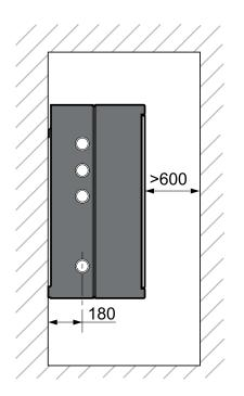
${\tt NOTE: All\ measurements\ are\ millimetres.\ Clearance\ necessary\ for\ the\ installation\ or\ maintenance\ of\ the\ appliance}$
