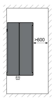
NOTE: All measurements are millimetres. Clearance necessary for the installation or maintenance of the appliance
