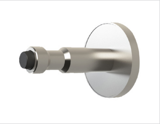
Coat hook 65mm Satin Stainless steel Stainless steel contemporary coat hook with concealed fixings and precision made groove retained buffer. Load tested to 30kg. Ø50 x D65mm Code: MFC / HPL / CC CH65T SGL CH65SG
