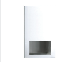
Elite warm air hand dryer Stainless steel Recessed mounted warm air hand dryer with brushed satin stainless steel cover and auto start/stop sensors. H579 x W382 x D116mm Code: 0302047
