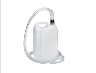
Plastic multi-feed soap dispensing system Multi-feed liquid soap dispenser for use with basin/vanity top, vessel basin or duct wall mounted soap dispensers with 5 litre refillable soap bottle. H283 x W190 x D130mm Code: 0362007
