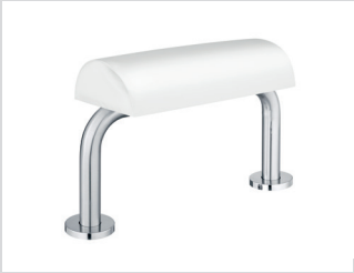
Back support rail Satin Aluminium back rest 400mm long with brushed satin stainless steel finish, concealed fixings and white vinyl pad. W400 x D310 x Ø35mm Code: S6466MY and S688467
