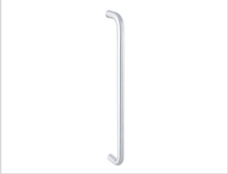
Door handle Satin anodised Satin anodised aluminium pull door handles. L400 x D45 x Ø19mm Code: Single 0182225 Pair 0182226
