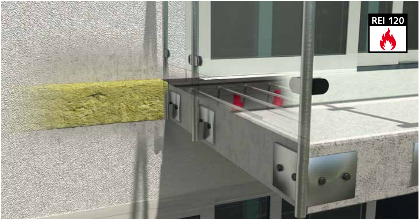
Installation example: HIT-HP and HIT-SP Elements, concrete to concrete connection
