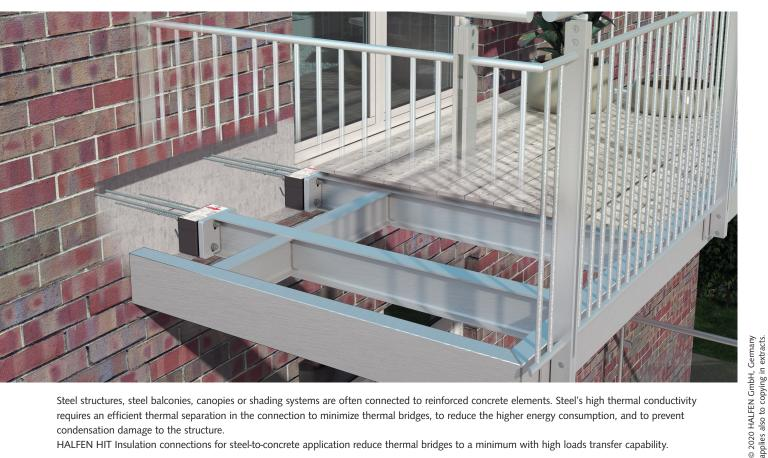
Steel structures, steel balconies, canopies or shading systems are often connected to reinforced concrete elements. Steel's high thermal conductivity requires an efficient thermal separation in the connection to minimize thermal bridges, to reduce the higher energy consumption, and to prevent condensation damage to the structure.
