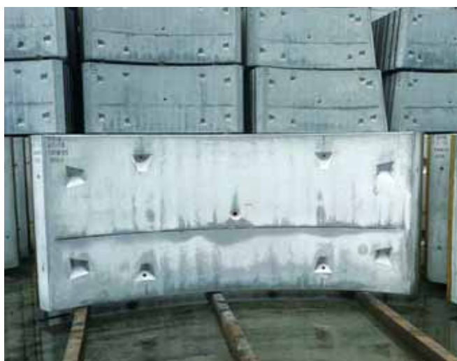
HALFEN HZA 29/20 Channels cast into tubing segments
