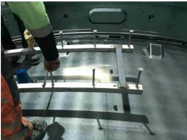
Fixing HALFEN Cast-in channels to the formwork for a tubing segment using HFK Fixing cones
