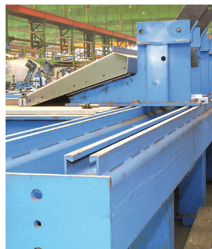
Welding-jig, locomotive construction
