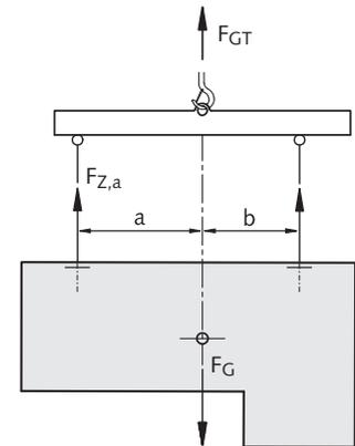
The load's centre of gravity will always stabilise vertically under the crane hook. Load distribution in non-symmetrically installed anchors when using a spreader beam is calculated as below:
