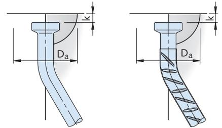
After installation the anchor head is near the centre axis of gravity. To ensure safe load anchorage the anchor foot is located in the centre of the support layer. This allows near vertical lifting and installation.
