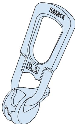
The DEHA Universal head lifting link is used for lifting and transporting precast concrete elements with cast in spherical head anchors. The universal head lifting link is a manual-release link. The universal head links currently available are Chrom-6-free zinc galvanized.
