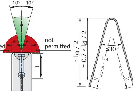
**i** Required reinforcement **4** only with diagonal pull → see table on page 22 "reinforcement in walls".
