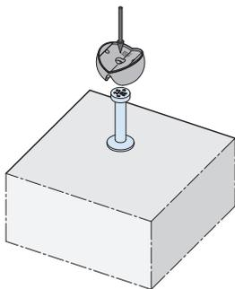
make a hole by removing a small amount of concrete with a trowel, place the recess former with the anchor in the hole.
