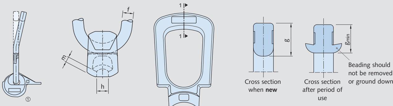
① It is prohibited to rebend any element damaged by misuse. Discard the universal head lifting link if there is any significant bending.
