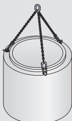
Three or four spherical head lifting anchors are used, depending on the size and weight of the element.
