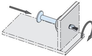
Loosen the screw or wingnut before striking the formwork.
