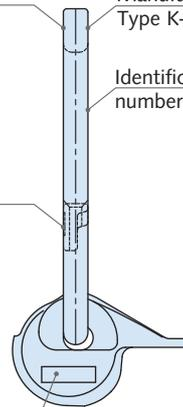
The application identifier K-A denotes that the universal head lifting link can be used for the following two DEHA Lifting anchor systems:
