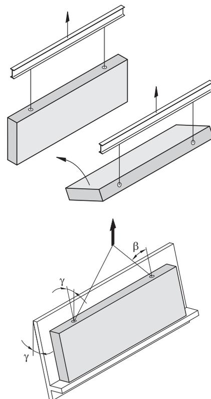
The transverse pull reinforcement can be omitted when using a tilting table and a load angle of  $\gamma < 15^\circ$ .
