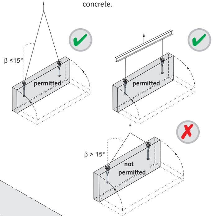
**!** The pitching anchor is permitted only for axial or transverse loading. Diagonal pull  $\beta > 15^\circ$  is not permitted. A spreader beam must be used when tilting with  $\beta > 15^\circ$ .
