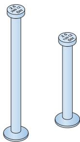
The load transfer into the concrete is via the anchor foot. This allows high possible loads with relatively short anchor lengths. In very thin elements these concentrated loads lead to lateral spalling caused by high tensile splitting.
