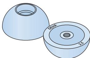
Magnetic steel recess formers are used in metal formwork when drilling is not an option.
