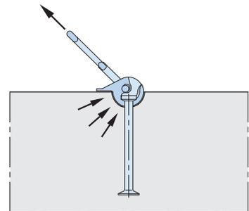
Consequently there is no reduction in load bearing capacity to account for diagonal loading in large surface elements. For example; as is standard for sleeve anchors. Additional reinforcement is not required.
