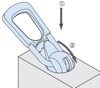
⚠ Turning is limited when the lifting link is under load.
