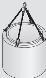
The lifting anchors can be installed in the pipe wall or in the tongue-end of the pipe.
