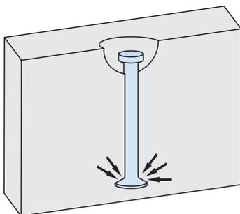
Compared with other lifting anchor systems the symmetrical design of the anchor foot does not require specific placement when installing the anchor (rotational symmetry).
