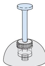
Slide the rubber grommet onto the anchor and press both into the hole in the steel recess former. If necessary, grease before use. Ensure the anchor is securely fitted and tied in place when the concrete is being poured.
