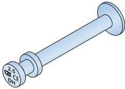
This DSM quick installation anchor can be used in situations where the recess former stays fixed to the formwork. This can be in face-up production of slabs, overhead production of utility pipes and installation in stair elements. Use a lubricant with the anchor to push into the DSM Recess former.
