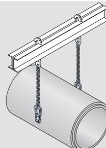
**Moving with two anchors in the hunches:**
