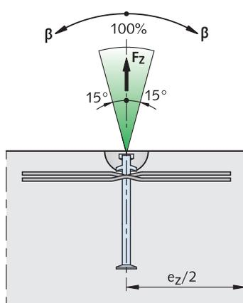
**i** Required reinforcement **1 - 3**. Pitching reinforcement is used instead of diagonal pull reinforcement → see table on page 22 "reinforcement in walls".
