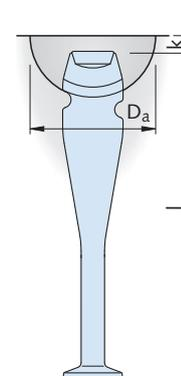
Dimensions of spherical head pitching anchors
