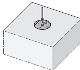
The concrete should be compacted until the upper surface of the former is flush with the surface of the concrete. To secure the anchor at the correct level, ensure that a plate (Art. No. 6141 or 6153) is inside the recess former. The anchors must be installed perpendicular to the surface. The use of formwork oil, especially inside the recess formers, eases removal and has a positive effect on the life span of the recess former.
