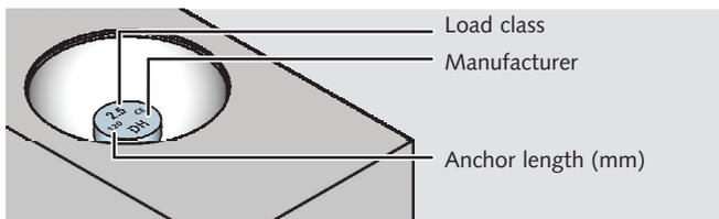
Maximal safety is only assured when using system components from only one manufacturer.
