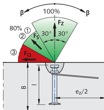
⚠ The slab has to be calculated for the load-case "lifting".
