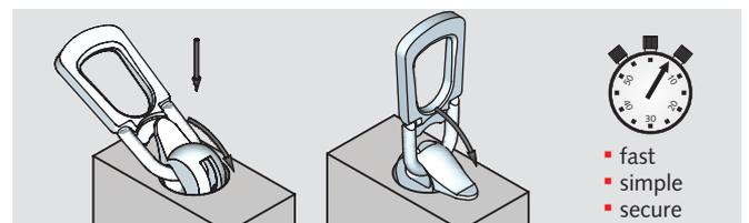
The only quick release lifting clutch capable of capacities from load class 1,3 to a maximum load class of 45,0 t.
