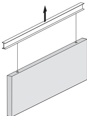
Diagonal pull lift  $\beta$ :  $10^\circ$  up to  $60^\circ$  ①
