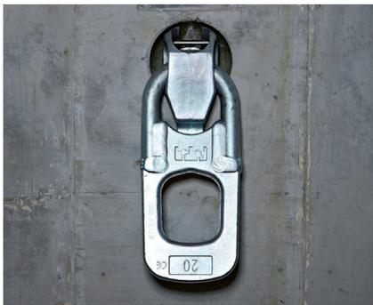
The HALFEN Recovery anchor system is a cast-in DEHA KKT Stainless steel spherical head lifting anchor, load class 20,0 on which a freely pivoting standard lifting link is attached. The lifting link is similar to the type used for moving precast concrete elements.
