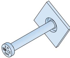
This anchor is recommended for all large surface, thin, precast elements that are lifted perpendicular to their main face (slabs and shell elements). This anchor can also be used in elements when the standard short spherical head anchor does not provide sufficient anchorage.
