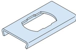
A steel pitching plate is required to avoid concrete spalling when lifting or pitching horizontally cast thin wall and ceiling slabs to the vertical.
