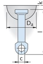
Dimensions of spherical head eye anchor
