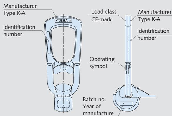
As with all lifting links, the universal head lifting links must be checked by suitably trained personnel at least once a year to ensure they are in a safe, usable condition. There is no pre-defined life expectancy for universal head lifting links.
