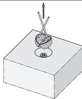
There are two holes in the recess former to help prise it out of the hardened concrete. Two reinforcement bars can be inserted in these holes and crossed against each other to open and remove the recess former. Excess concrete should be removed.
