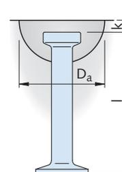
Dimensions of spherical head anchors
