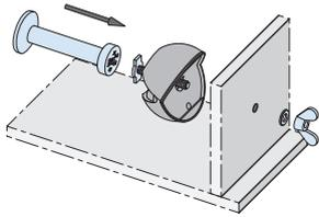
The recess former is subsequently attached to the formwork with a screw or with a wingnut.
