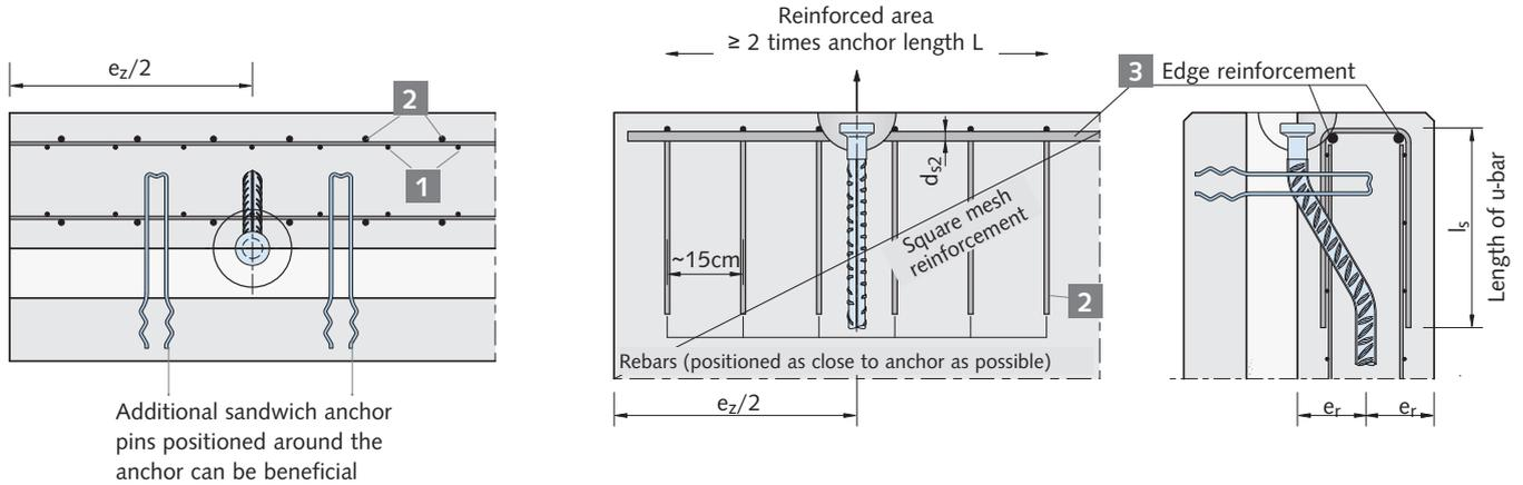
Reinforcement and load capacity of spherical head anchor; offset type with axial pull  $< \beta = 30^\circ$
