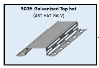
Galvanised top hat profile. 0.9mm gauge 26mm x 27mm x 60mm x 27mm x 26mm 3 metre lengths
