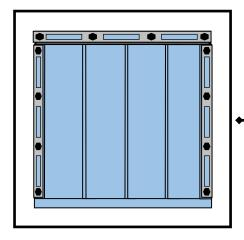
Place the universal carrier trim over the existing fixings and screw into the flat areas in between the cut outs until you are sure of a positive fix.
