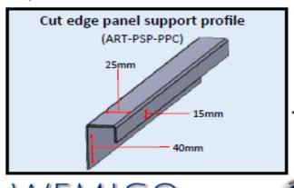
Aluminium support trim used with a cut edge panel for edge support. Or ventilated to use as a starter trim for vertically laid planks.
