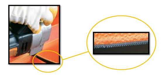
DO NOT use a hack saw or abrasive disc as these can leave an uneven, poorly finished cut. These methods also cause frictional overheating and abrasion which can damage the coating.
