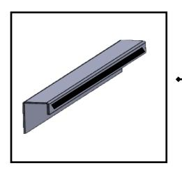
If a plank has to be cut along its length it is necessary to install a cut edge panel support profile under the cut end. This is installed before the panel is fixed into place. This trim, when it has been perforated, is used as a starter trim for vertically installed systems. When using as a cut plank support, use a strip of Wemibond tape to bond the panel and create a seal before fitting the cover trim.
