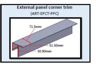
Aluminium cover trim used vertically left or right, or as a header and base trim for cut or complete panels.
