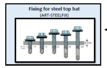
Bi metallic hexagon head self drilling screw for securing panel to timber purlins. Coated carbon steel and Austenitic stainless steel A2 (304grade) 6.3 x 50mm S16 washer
