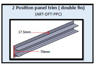
Aluminium support trim used with a cut edge panel for edge support
