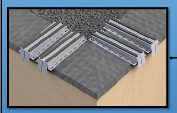
Using a plumb-line, lay out the brackets onto the parapet to establish the optimum positioning. Always allow two brackets per corner leg and a space at 720mm centres along the remainder of the parapet. Brackets must be kept clear of the locations of joins between successive coping lengths, so they do not clash with the joining pieces.
