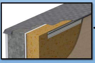
Place the Wemflex vapour barrier along the parapet ensuring an even amount overhangs each side to ensure a weathertight seal can be created.
