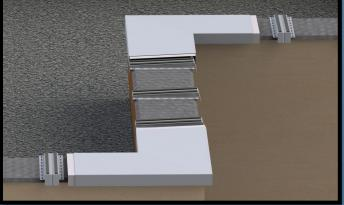
Snap the corner pieces into position first over the previously installed retention brackets.
