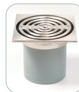
ADV/SS/150S Caroflow 150mm Square Stainless Steel Advantage Trapped Grating Assemblies suitable for use in tiled flooring situations and simple connection to 110mm socketed pipe.
