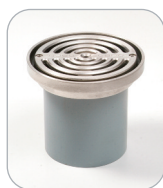
ADV/SS/150C Caroflow 150mm Circular Stainless Steel Advantage Trapped Grating Assemblies suitable for screeded floor finishes and simple connection to 110mm socketed pipe.
