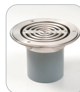
ADV/SS/150CF Caroflow Stainless Steel Advantage Trapped Grating Assembly with Clamping Flange. Suitable for use in vinyl/sheet flooring situations and simple connection to 110mm socketed pipe.
