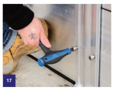
The horizontal screws can now be tightened. DO NOT OVER TIGHTEN.
