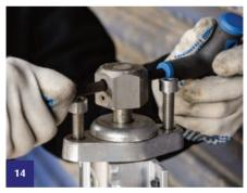
Now fully tighten Demountable Post hexagon bolt using the T-Bar tool through it.
