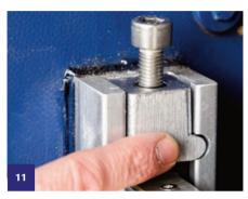
Insert compression block into fixed wall post and finger tighten.
