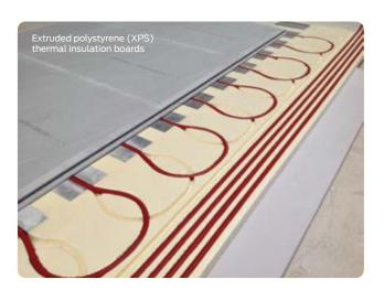
This system relies on the floor being flat and level and involves pre-grooved polystyrene floor insulation panels, fitted with pre-grooved metal diffusion plates into which the underfloor pipework is fitted.
