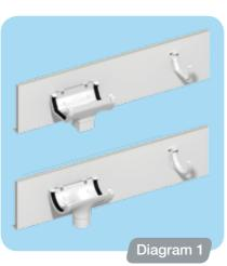
The procedure for gutter fixing is dependent upon the design chosen, i.e. End or Centre Outlets for houses with standard gable ends, and a combination for hipped roof buildings. In all cases the Outlets should be positioned directly above the gully or drain connection if at all possible. Before installation, check that fascia boards etc. are level, and make allowances if not, when determining gutter fixing positions.
