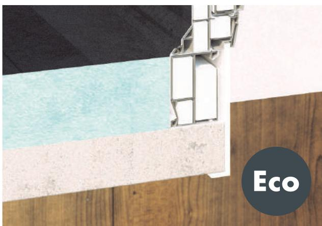
Profiles are filled with insulation material, thus additionally improving the energy saving parameters of the product. The specially profiled covering material under the frame drip cap further improves the ultimate finish between the window and the roof covering.
