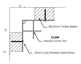
Fit corner trims to all Internal (CL006) and External Corners (CL005) as shown fixing with 25mm stainless steel screws at 300mm centres. The Corner Trims must pass beyond the bottom of the first cladding board when fitted, the Corner Trims should run 12mm past the bottom of the Starter Bar (CL001).
