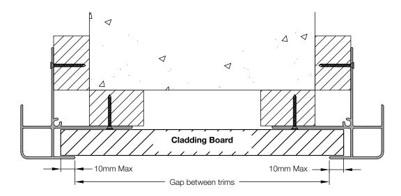
The cladding board cut length should be a maximum of 20mm longer (10mm per side) than the gap between the aluminium trims. Shorter board lengths may require the 10mm per side to be reduced to ease fitting and enable the board to shuffle into position rather than bend.
