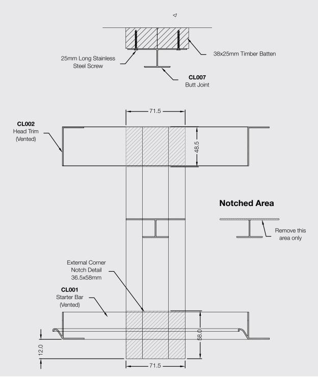
Where a butt joint is required, 2 vertical timbers are required to allow the butt joint to be fixed. Using stainless steel screws fix at 300mm centres. For the Butt Joint (CL007) to run full length the back section of the Trim must be notched out where the Starter Bar (CL001) and Head Trim (CL002) run through.
