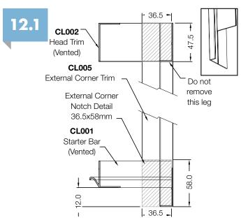
**End Closer Notching Details:-** To allow the Starter Bar (CL001) and Head Trim (CL002) to run full length, notching is required on the End Closer (CL004)
