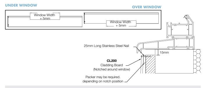
If cladding runs around a window, boards may need notching around the window at both the top and bottom. The size of the notch is dependent on the window size and where the stacked boards locate. Overleaf is an example of possible notching details for both over and under the window. A packer may be required behind the notched board to aid fixing.
