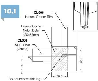
**Notching Details:-** To allow the Starter Bar (CL001) to run full length, notching is required on the Internal (CL006) Corner Trims. Cut away the section shown below.
