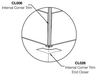
Where Internal and External Corner Trims (CL005 & CL006 are used, screwported End Closers (CL025 & CL026) are available. These are to be fitted by offering up to the end of the corner trim and screwing into the screw port in the aluminum extrusion.
