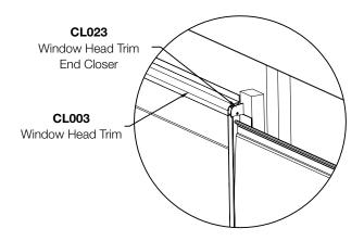
Window Head Trims (CL003) require to be capped off to create a neater finish, Window Head Trim End Closers (CL023) are available. Fix the End Closer to the Window Head Trim by screwing through the End Closer into the screw port in the aluminum extrusion.
