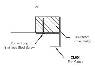
Locate the End Closer (CL004) onto the timber batten, fix using 25mm stainless steel screws. The End Closer (CL004) must be long enough to pass beyond the bottom of the first cladding board when fitted, the End Closer (CL004) should run 12mm past the bottom of the Starter Bar (CL001).
