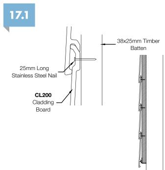
Once secure stack the next cladding board by hooking over the top lip which hides the fixings, as before fix back to the timbers through the to section of the cladding board. Continue this method until the cladding is complete.
