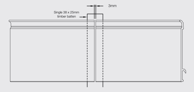
An alternative method of jointing the Cladding Boards is to butt the boards together leaving an expansion gap of 3mm between the adjoining boards. With this option a single timber batten at the join location should be used. Apply 'lead alternative flashing' to the timber behind the joint to protect the timber from any water that penetrates the expansion gap. Care should be taken when fixing the board to the single timber batten so as not to split the board by excessive use of force.
