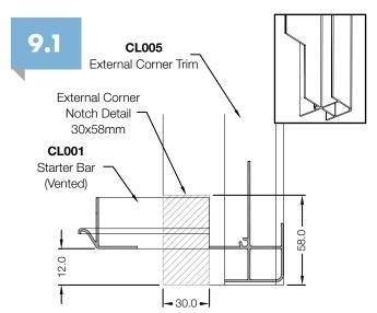
**Notching Details:-** To allow the Starter Bar (CL001) to run full length, notching is required on External Corner Trims (CL005). Cut away the section shown below.
