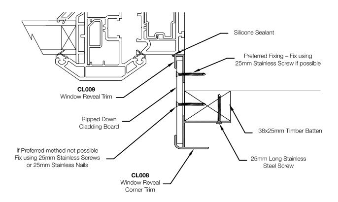
The Window Reveal Trims (CL008 & CL009) and Window Head Trims (CL003) need to be fitted before installation of the cladding board begins. This is to allow the trims to be fixed correctly.
