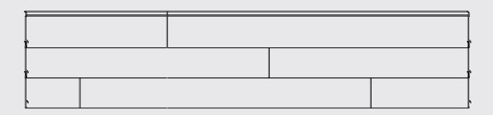
Stagger the joints on each cladding level to give a more aesthetically pleasing finished look.
