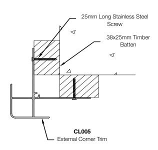
Fit corner trims to all Internal (CL006) and External Corners (CL005) as shown fixing with 25mm stainless steel screws at 300mm centres. The Corner Trims must pass beyond the bottom of the first cladding board when fitted, the Corner Trims should run 12mm past the bottom of the Starter Bar (CL001).
