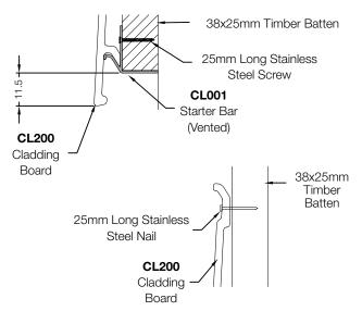
To begin the installation of the coastline cladding boards, locate the first board onto the Starter Bar (CL001), fixing at the top using 25mm stainless steel nails fixing back to each timber batten (max 500mm centres).
