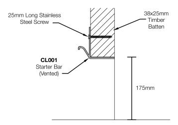
Once the window reveals have been completed fit the Starter Bar (CL001) to the bottom of the timbers, fix back to each batten as shown using 25mm stainless screws.
