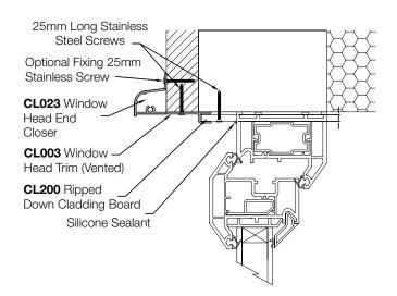
Cut down a section of cladding board to the required size. Position the board into the Window Head Trim (CL003) and fix head trim up into the timber battens using 25mm stainless screws. Once in position fix the board up into the brickwork and seal the end with a silicone sealant.
