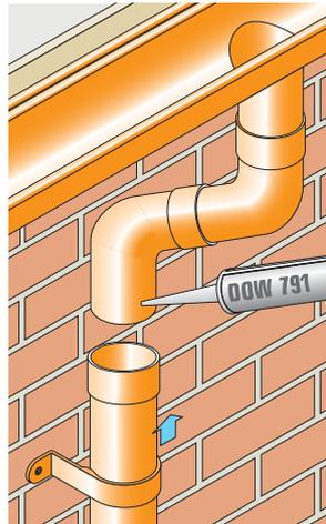
Commence installation from the gutter outlet by fitting and adjusting the two part offsets. Check vertical plumb line and assemble swaged joints using DOW 791 silicone sealant then fit first pipe clip.
