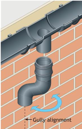
Where square or rectangular pipes are being installed and offsets are required, alignment between the gutter outlet and gully must be exact. Round pipe systems are more flexible to install and offsets can be adjusted and “swung” into alignment with the gully position.
