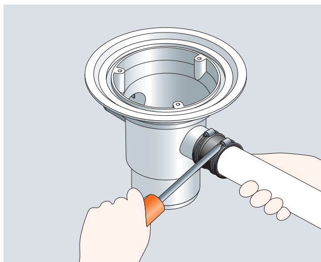
2. Insert plain end of 50mm waste pipe into coupling. Tighten screws on metal strap to secure.
