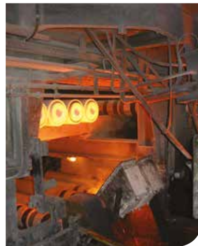
Centrifugal casting process
