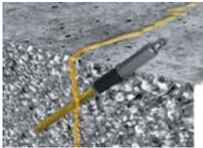
WATERPROOFING OF CONSTRUCTION JOINTS
