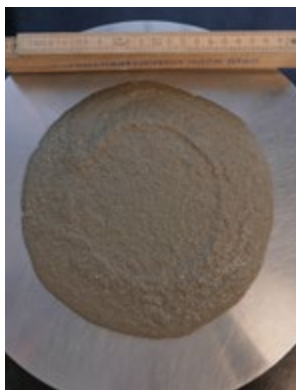
Standard mortar without SikaGrind®
