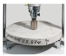
Round panel test: ASTM C1550
