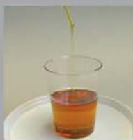
Due to the low viscosity of Sika® Injection-201 it can penetrate into cracks >0.2 mm in width.
