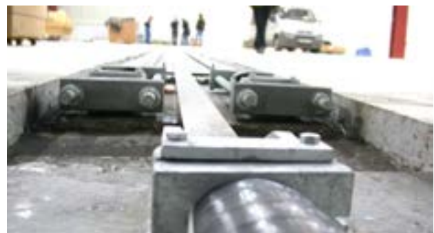
Base channel with post-tensioned CFRP plates
