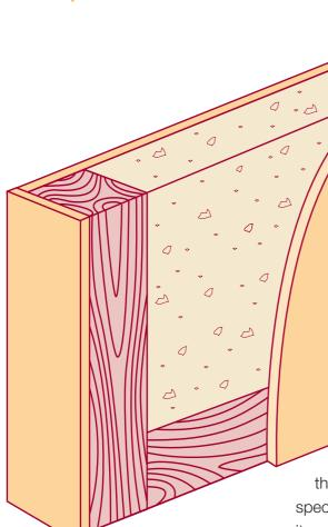
The Series 2 is a genuine 100% solid timber and high density flaxboard core flush door. Due to the fact that
