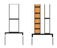
Where the external face of the wall is at or near to the edge of the foundation block, it is sufficient to ensure that the vertical centre line of the wall is within the middle third of the foundation width.
