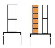
Where the external face of the wall is at or near to the edge of the foundation block, it is sufficient to ensure that the vertical centre line of the wall is within the middle third of the foundation width.
