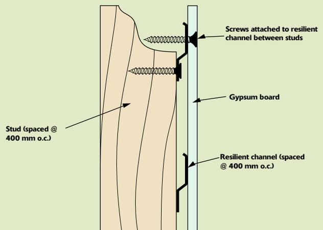
*The screws used to attach the gypsum board to resilient channels must be located away from the studs, as any direct contact with structural members would create a path for sound transmission.*
