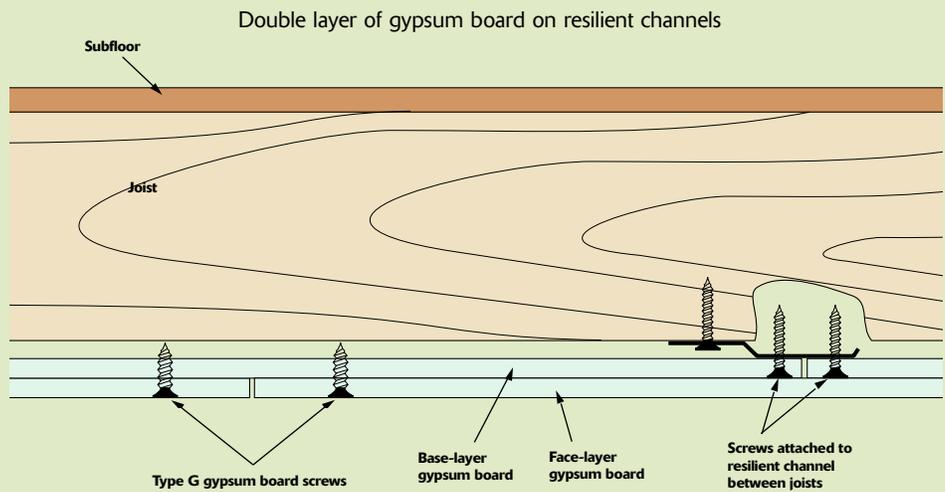
*The screws used to attach the gypsum board to resilient channels must be located away from the joists, as any direct contact with structural members would create a path for sound transmission.*
