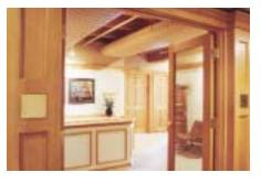
The surface appearance and easyworking properties of Douglas fir are appropriate to the manufacture of window and door frames, mouldings, cabinets and other joinery. The hardness and strength of Douglas fir add the dimension of durability.
