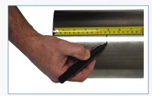
**2.** Measure and mark required depth on the tube using a tape measure and marker pen.
