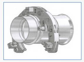
**10.** Open the mouth of the sling and slide the sling down the fitting until the wheel guides are sitting against the end socket of the fitting.
