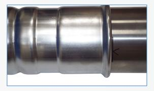
**4.** Insert the tube into the fitting until it meets the fitting stop and check that the line and 'V' marking is visible.
