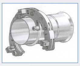
6. Open the collar and place it on the bead of the fitting (the collar joints are spring pre-loaded). Make sure that the wheels are positioned on the tube side of the fitting.
