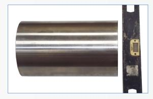
**1.** Cut tube square to the required length using a fine tooth electric saw and deburr the outer and inner end in order to prevent any damage to the O-Ring.
