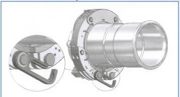
8. Attach the press tool to the mouth of the fitting - use the handle at the top of the press tool to open the jaws on the adaptor. Swivel the catch inwards and secure the lock. The claws of the adapter jaw must be firmly gripped onto the press collar.
