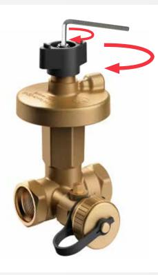
An Allen key is used for differential pressure setting of the Ballorex Delta. The black handle enables flow isolation.
