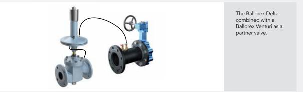
When the Ballorex Venturi is used as a partner valve and installed in the supply line, it is within the circuit controlled by the Ballorex Delta. In this case the pressure loss across the Ballorex Venturi valve adds to the pressure loss in the controlled circuit and needs to be taken into account when setting the Ballorex Delta valve.
