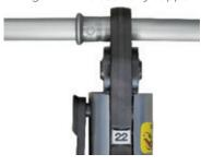
pipework, and with your hands safely away from the joint, press the trigger or button to start the jointing cycle. When the jaws/sling jaws fully enclose the mouth of the fitting, the joint is complete. The jaw should
