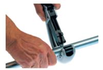
The tube must always be cut completely. Never partially cut and then broken as this could cause corrosion. Do not use hacksaw, oil cooled saws, abrasive wheels or flame cutting.
