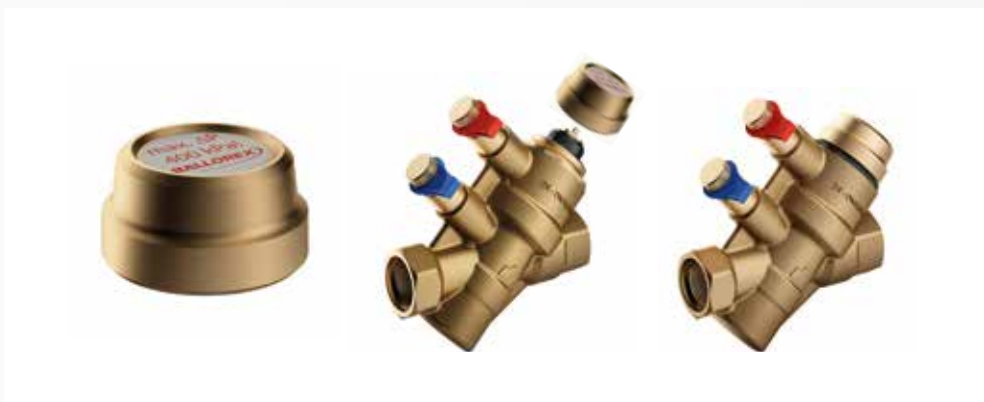
The shut-off cap is used for flow isolation across the Ballorex Dynamic valve provided that the differential pressure across the closed valve never exceeds 400 kPa. Index
