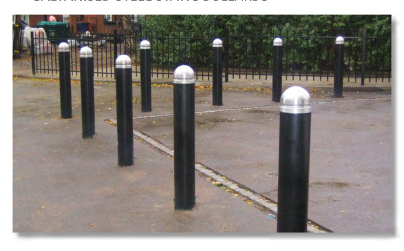
Ideally suited for demarcation and commercial use to prevent vehicle entry and segregation of pedestrians and vehicles the galvanised bollards can be supplied heavily galvanised to BS EN 1461 or have an additional paint finish either polyester powder coating for normal environments or marine coat for coastal or hazardous situations.
