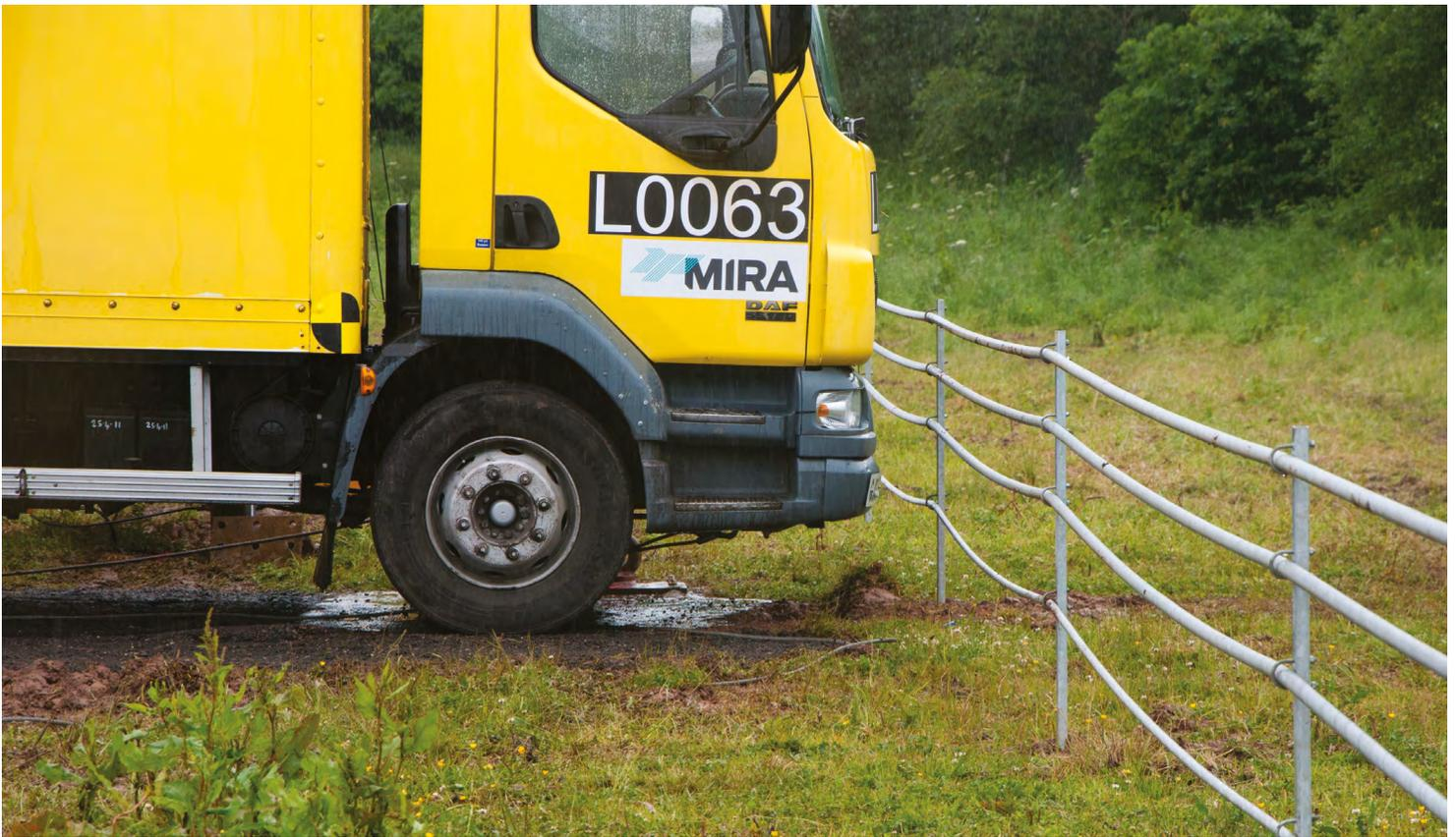
The Jacksons Linebacker® is a cable crash fence and gate system has been successfully impact tested in accordance with BSi PAS 68:2010 for the performance of vehicle security barriers and their supporting foundations when subject to a single horizontal impact.
