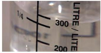
5. Mix the mortar with exactly 30 ml of water. Add the water to the supplied container and mix with the dry mortar
