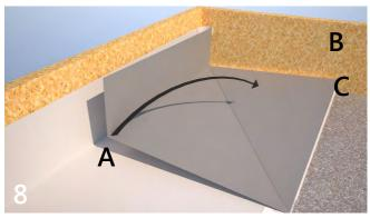
Holding the membrane at point A of the grey flap and fold back so that your hand is at point C. The upstand B of figure 7 should now be against the formwork at point B. At this stage only the white fleece should be facing upwards.
