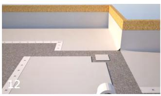
For external corners, cut a square of membrane and from a corner of that square, cut out a small square of about 75mm x 75mm. Fit the square to the corner and when in place, tape the square under the membrane already in place.
