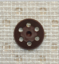
Newton damp proof membranes have a pattern of raised studs which create air channels to enable the damp wall to dry out
