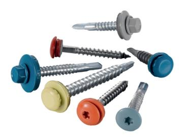
SFS offer fasteners in a range of materials with different levels of corrosion resistance. Carbon steel could typically be warranted up to 12 years, A2 (304 grade) austenitic stainless steel for up to 25 years and A4 (316 grade) austenitic stainless steel for up to 40 years. For more guidance on the selection of fastener materials please refer to SFS's "Designers Guide" or consult our Specification or Technical Teams.
