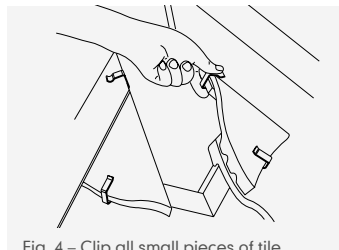
Fig. 4 - Clip all small pieces of tile along hip
