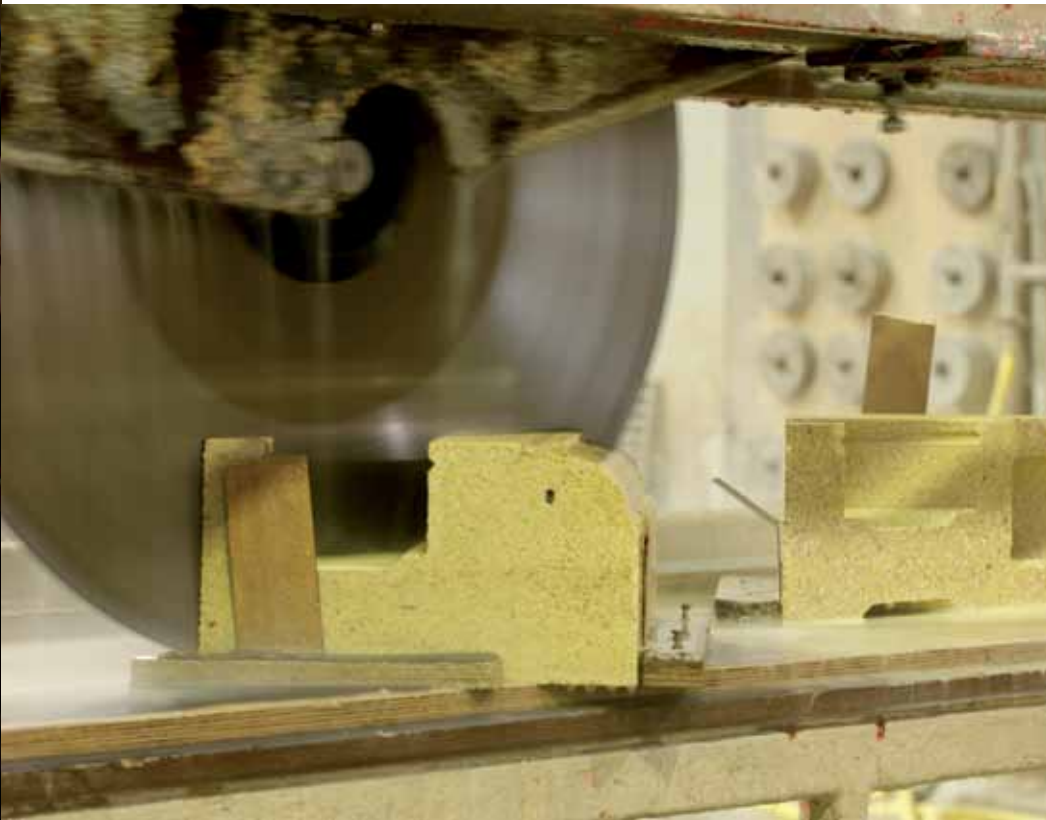
Diamond headed masonry saw slicing through Roof Block
