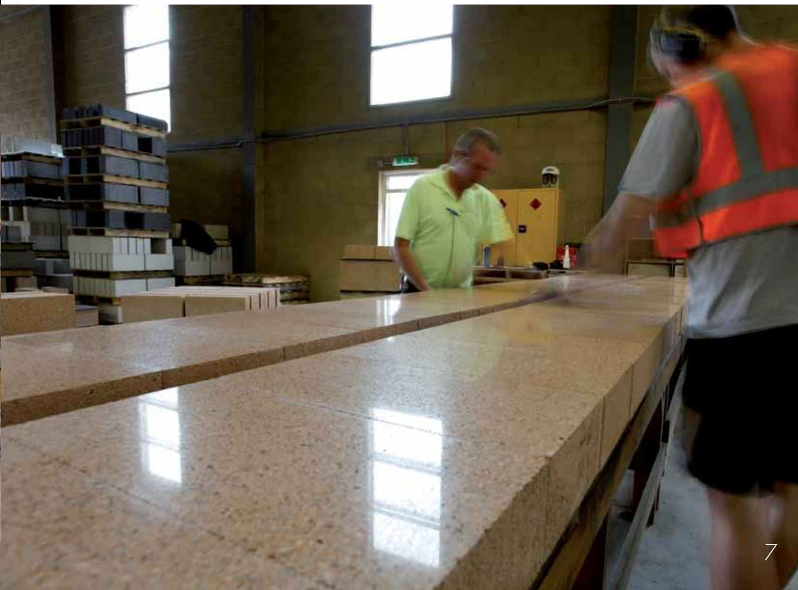
Polished masonry being hand finished.
