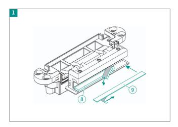
The hinge is pre-assembled for 8 mm thick door leaves. For 10 mm thick door leaves, remove the intermediate layer ® without leaving any residue and glue in the intermediate layer ⑨.
