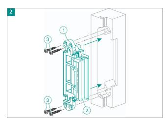
Place the hinge frame part 1 in the door frame, pre-drill the door frame and fasten the hinge frame part with the four screws 3 (4.5x30 mm).
