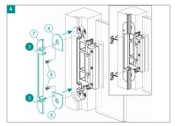
Fasten the cover plates 4 and 5 to the hinge with the screws 6. Fasten the rebate cover 7 with the two screws 3 flush to the frame on the cover plates. Cut the door seal to size.
