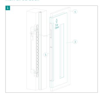
Clean the adhesive surface on the glass door  $\ensuremath{\mathfrak{4}}$  with the enclosed cleaning cloth.
