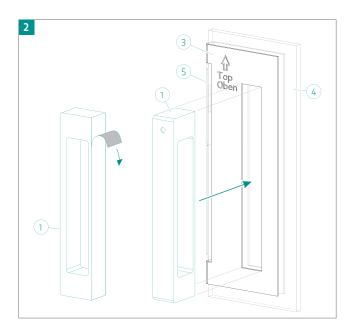
For assembly, put the KC Lock handle with locking function  ${\bf 1}$  in the locked position.
