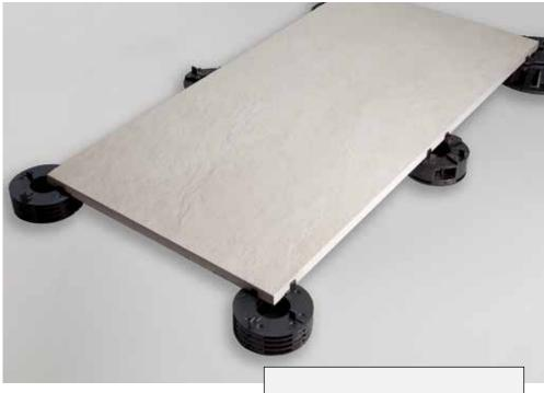
10 tile and paver supports. As up to 10 x Schlüter<sup>®</sup>-TROBA-LEVEL-PL 30 adapter blocks can be stacked together this means they can be used to create an assembly height of between 50 and 320mm.
