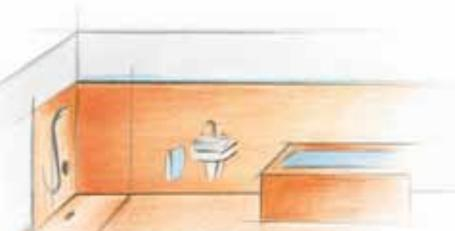
Areas in showers, behind sinks and around baths are considered wet areas with high moisture loads that can be protected effectively with the bonded waterproofing membrane, Schlüter®-KERDI.
