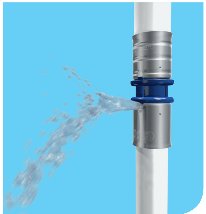
Figure 4: Safety through clever technology: the Defined Leak Function in the pressure test reveals unpressed fitting connections
