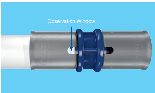
Figure 2: The observation window in the stainless steel press sleeve can be used to check that the pipe is inserted to the stop
