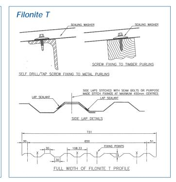
Recommended purlin and vertical rail centres 1m. Note that, although shatter resistant, Filonite is flexible and must not be stood on when on the roof. It is recommended that a sealing tape is used at side lap positions as illustrated.
