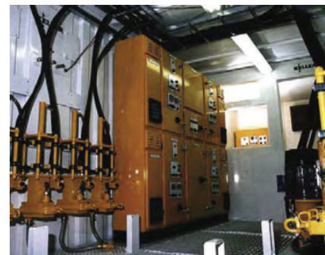
Compensation Grouting module and control centre.
